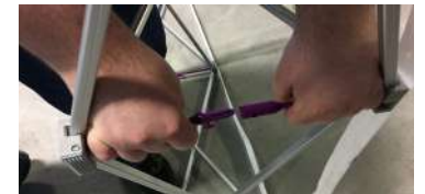
3A. Make contact when lining up the female arm and the frame hub for easier connection.
