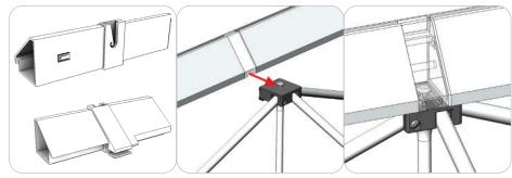
The back-lit scissor frames will have middle hubs with a metal prong installed on all four sides front and back. Attach the middle caps of the back-lit channel bars onto the middle hubs. The middle caps of the channel bar will snap into place.
